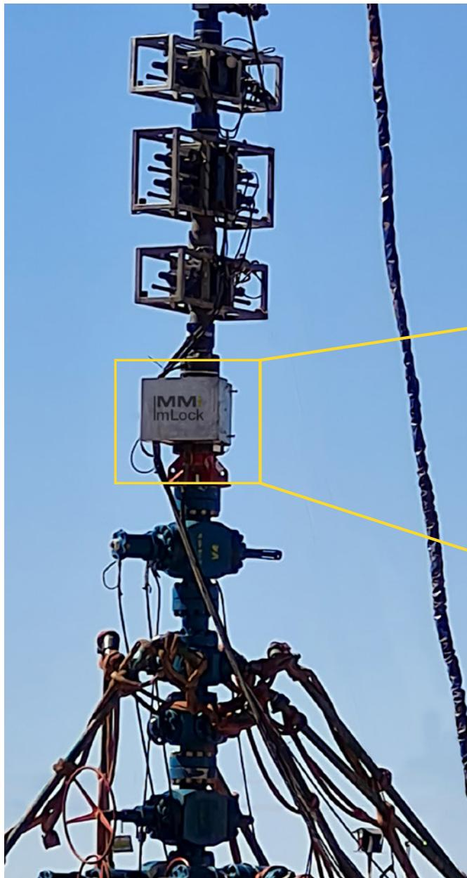
mLock is a remote hydraulic connector for wireline operations. It allows the wireline equipment to be connected to the well quickly and safely. It has a control system that provides the process logic with guaranteed safety for performing operations.
